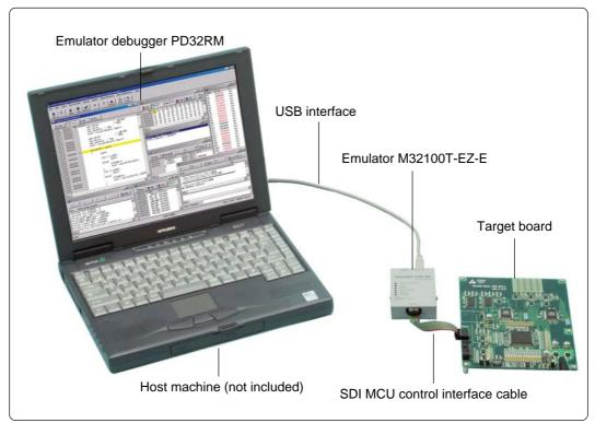
Figure 2.1 System configuration (JTAG connection)
